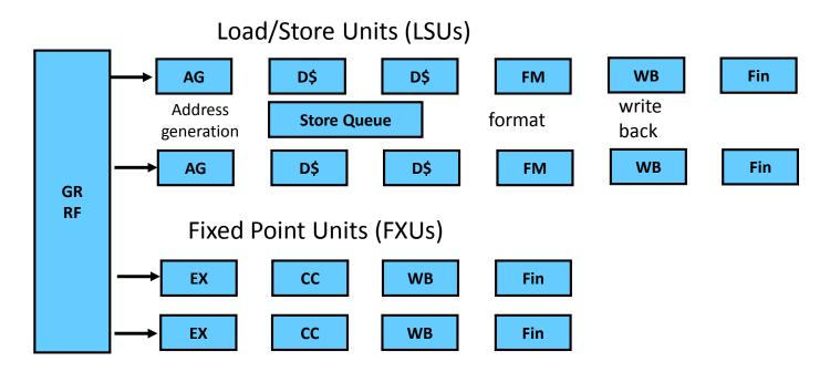
Depiction of part of the z196 pipeline showing 2 load/store units and 2 fixed point units. The stages for instruction fetch, decode and grouping and putaway are not shown. Also not shown are the floating point units for binary and decimal arithmetic. Under ideal conditions, the z196 can execute 5 instructions simultaneously.
