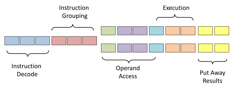
Each box from left to right represents a pipeline stage which takes one cycle. After instructions have been decoded and put into superscalar groups, they are issued down the two pipes one or two instructions at a time. In this example, the apparent order of execution is still maintained.
