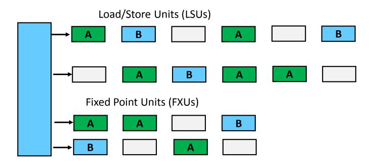
Each stage of the pipeline can process an instruction from thread A or an instruction from thread B or no instruction. Pipeline bubbles for one thread can be filled with instructions from the other thread.
