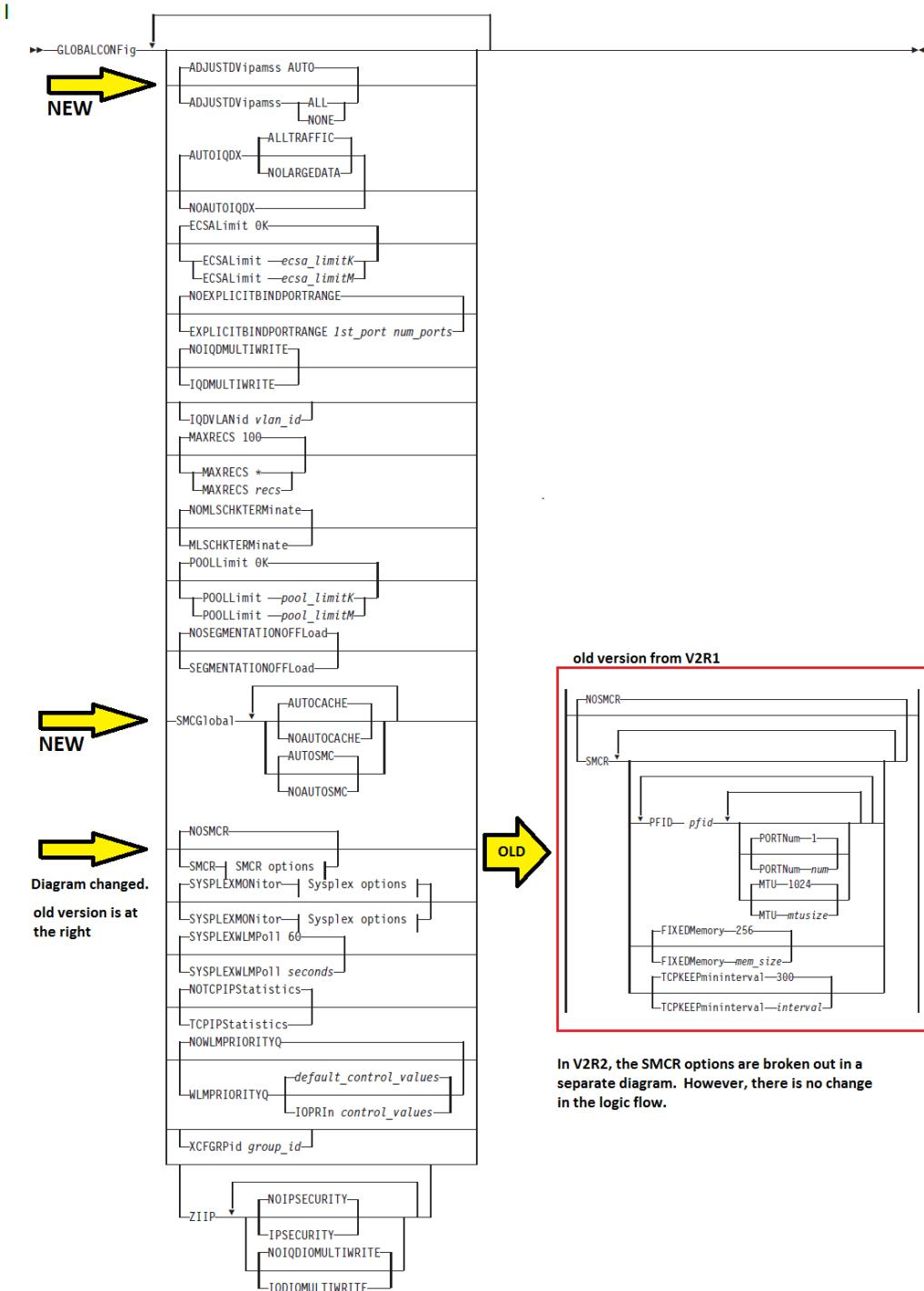
In V2R2, the SMCR options are broken out in a separate diagram. However, there is no change in the logic flow.
