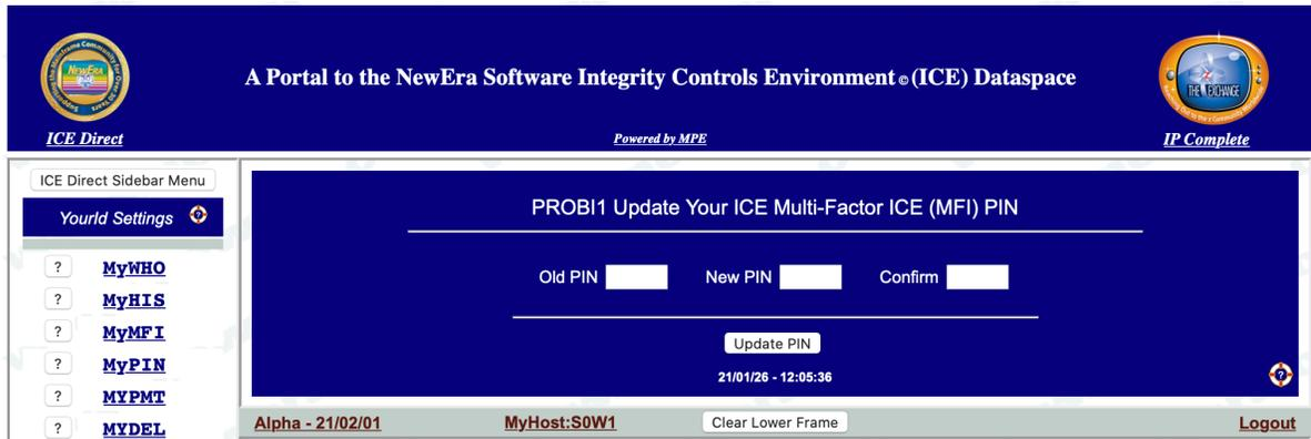
This specific panel is the Interface Panel for the “MyMFI”. Use this panel to update the Prefix/PIN used to authenticate with ICE and Login to ICEDirect. Selecting the “Life-Ring” in the lower right will display the Help Panel Floater shown in part below:
